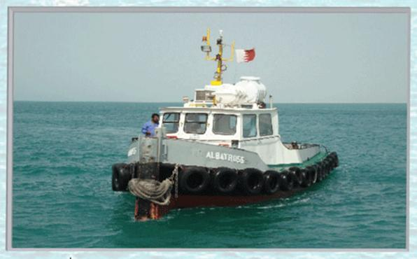
"ALBATROSS" NAME CALL SIGN AD3054 LENGTH OVERALL **44.8 FEET** BREADTH OVERALL 14.0 FEET DEPTH **5.20 FEET** DRAFT GROSS TONNAGE 20.04 TONS PORT OF REGISTRY / NO. **BAHRAIN / 8530** FLAG BAHRAINI PLACE & YEAR BUILT U. K. - 1974 REBUILT 2010 CLASS A.M.S.
