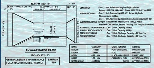
The aft and forward of this ro-ro barge are fitted with hydraulic adjustable ramps, capable of transporting any heavy equipment from port to port, ship to ship and to any harbour according to the height of harbour. Also capable of loading and unloading from a sand beach and to any Island in Gulf.
