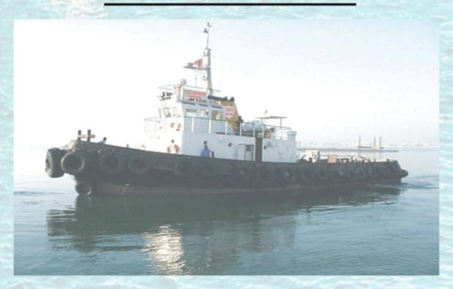
NAME "MANAR" LENGTH OVERALL 88.77 FEET BREADTH OVERALL 26.76 FEET DEPTH 15.51 FEET DRAFT 13.86 FEET **GROSS TONNAGE** 164.7 TON
