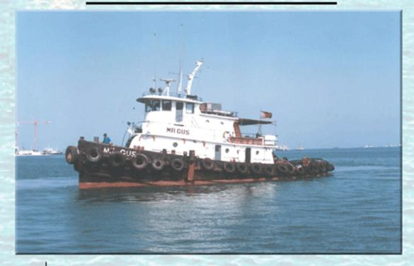
"MR. GUS" A9D 2008 NAME CALL SIGN LENGTH OVERALL 75 FEET BREADTH OVERALL 24 FEET DEPTH 11 FEET DRAFT 9 FEET **NET TONNAGE 59 TONS GROSS TONNAGE** 87 TONS PORT OF REGISTRY / NO. BAHRAIN / 2080 FLAG BAHRAIN PLACE & YEAR BUILT U. S. A. - 1965 REBUILT **BAHRAIN - 2003**
