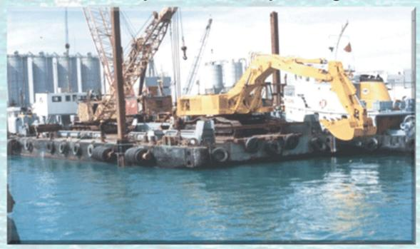
NAME "RAZAN" LENGTH OVERALL 115 FEET BREADTH OVERALL 36 FEET DEPTH 10 FEET DRAFT 5 FEET **NET TONNAGE** 283.27 TONS **GROSS TONNAGE** 283.34 TONS **425 TONS** D. W. T. PORT OF REGISTRY / NO. BAHRAIN / 1089 BAHRAIN FLAG **DECK CARGO AREA** 82 FT. X 32 FT. ACCOMODATION 4 PEOPLE PLACE & DATE OF BUILD **JAPAN - 1977** REBUILT BAHRAIN - 2003
